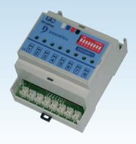
Output card for controlling 1 to 8 500 or 1000 W dimmers or module 0-10 V  $\,$  1-10 V.
