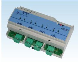
Control card with from 1 to 4 3 channel outputs. For controlling valves, motors, shutters, etc., consists of 8 250 V-8 A relays.
