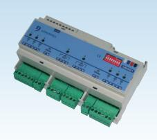
Output card to control 8 250 V/8 A two-pole relays. The card is fitted with a micro-switch to select the relays which can be controlled by a switch without the presence of the Master. Connection of the Bus is by means of a rapid 4x4x1 mm<sup>2</sup> connector.
