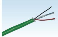
The bus cable contains 4 conductors of which two (black and red) are 0.75 mm for powering the modules at 12 V DC and two (white and blue) form a 0.28 mm twisted pair for data.
