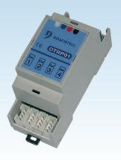
Output card for the control of 1 to 4 trip switches. Currently reserved for the connection of trip switches marketed by our company. Several cards can be connected.
