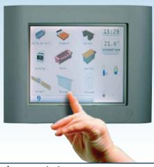
Back-lit touch screen for the display and control of home automation points and the setting of certain functions (temperatures, clocks, etc.).
